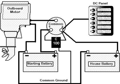
supplied from the starting battery in position 1 but battery 2 or both can be selected in an emergency. In all cases, both batteries are being charged when the engine is running. WARNING: If you use this circuit, turning the switch to "OFF" while the engine is running may damage your alternator.
